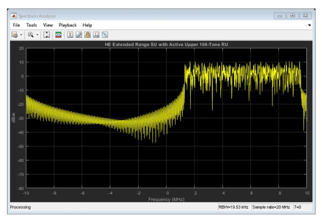
If we compare the power of the L-STF and L-LTF fields we can see the extended range transmission is boosted by 3dB.
