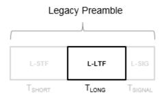
Channel estimation, fine frequency offset estimation, and fine symbol timing offset estimation rely on the L-LTF.
