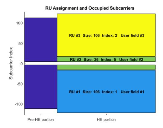
The ruInfo method provides details of the RUs in the configuration. In this case we can see three users and three RUs.
