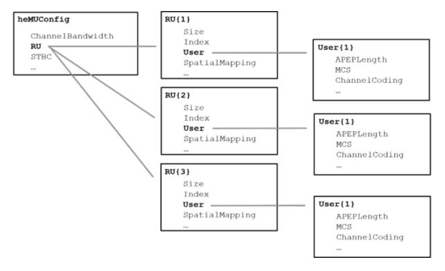
In this example, three RUs are specified by the allocation index 128, therefore cfgMU.RU is a cell array with three elements. The index and size of each RU are configured according to the allocation index used to create cfgMU. After the object is created, each RU can be configured to create the desired transmission configuration. For example, the spatial mapping and power boost factor can be configured per RU. For this configuration the first RU is RU# 106-1 (size 106, index 1).
