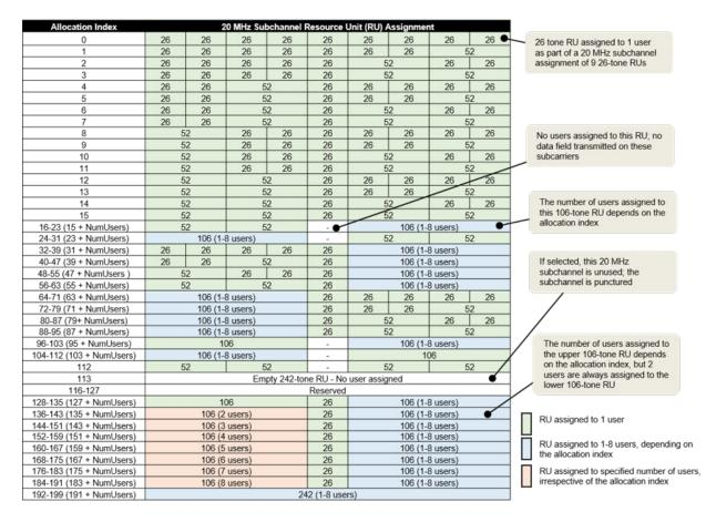
The RU allocation and HE-SIG-B user signaling for allocations > 20 MHz is shown in the table below, with annotated descriptions.
